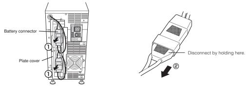
**3.** Turn the 2 screws that fix the plate cover anti-clockwise to remove them. ① While pulling the plate cover toward you ②, lift it up and remove the lower battery connector from the eyehole.
